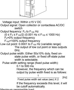
Maximum permissible load: Open collector: 30 V DC/200 mA Contactless AC/DC Switch: 240 V AC/200 mA Zero adjustment: ±1% Span adjustment: ±1%
